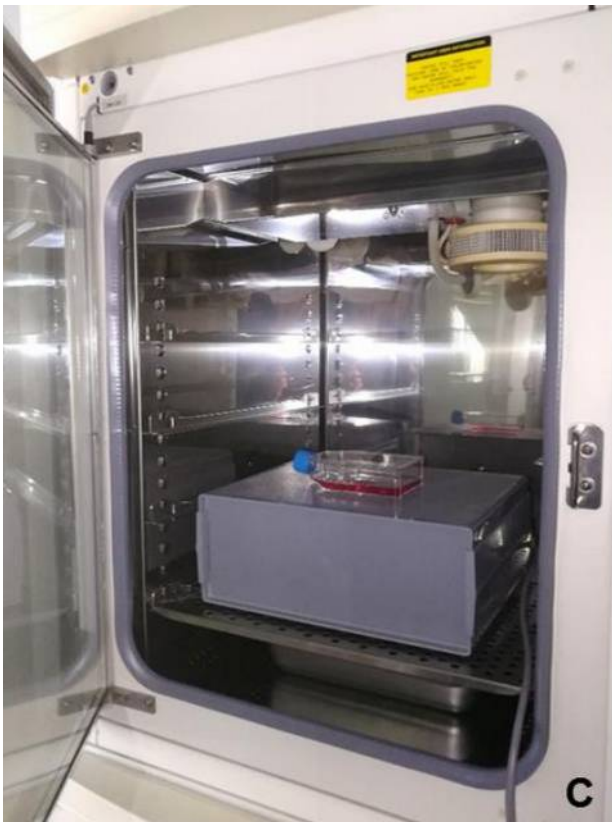
Fig. 18 - Photo of the antenna enclosure housed inside a 37^\circ\text{C} , \text{CO}_2 controlled incubator for experiments.
